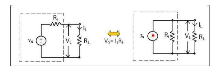
R1's in figure represents the internal resistance of the voltage source VS and current source IS.
