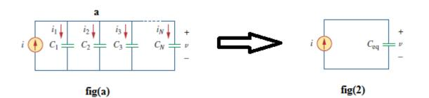
Applying KCL to the circuit in figure (a) we can write: i = i1 + i2 + i3 + ....+ in.....(1) i = C1 (dv/dt) + C2 (dv/dt) + ... + Cn dv/dt) = (C1 + C2 + ... + Cn) (dv/dt).....(2)Similarly for the circuit in figure (b) we can write the governing equation as: i = Ceq (dv/dt).....(3)From the eq(2) and eq(3),we get Ceq=C1+C2+....+Cn Note: The equivalent capacitance of a circuit consisting of n capacitances C1, CL2,....and Cn
