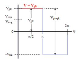
When plotted as voltage (V) as a function of phase ( $\theta$ ), a square wave looks similar to the figure to the above. The waveform repeats every  $2\pi$  radians (360°), and is symmetrical about the voltage axis (when no DC offset is present). Voltage and current exhibiting cyclic behavior is referred to as alternating; i.e., alternating current (AC). One full cycle is shown here.
