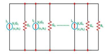
Let I represent the resultant current of the parallel current sources while G the equivalent conductance as shown in the figure below.
