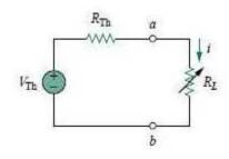
According to Maximum Power Transfer Theorem, for maximum power transfer from the network to the load resistance,  $\mathbf{R}_{L}$  must be equal to the source resistance i.e. Network's Thevenin equivalent resistance  $\mathbf{R}_{Th}$ . i.e.  $\mathbf{R}_{L} = \mathbf{R}_{Th}$
