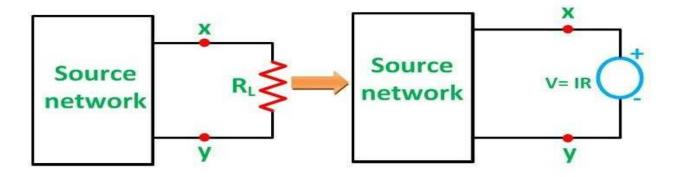
Let us assume a load  $R_L$  be connected to a DC source network whose Thevenin's equivalent gives  $V_0$  as the Thevenin's voltage and  $R_{TH}$  as the Thevenin's resistance as shown in the figure below.
