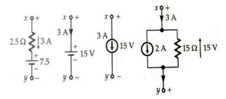
Figure: (b) Equivalent branches across terminals 'xy'
