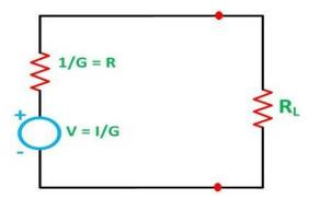
$$V = \frac{I}{G} = \frac{\pm I_1 \pm I_2 \pm \cdots \pm I_n}{G_1 + G_2 + \cdots + G_n}$$
