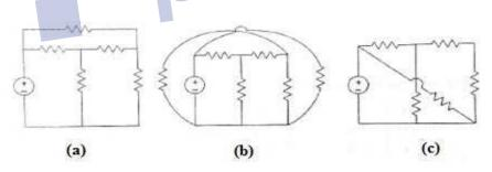
Loop: It is a closed path along the circuit elements.
