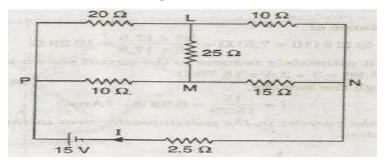
**Solution:** Delta connected resistors 25 ohms, 10 ohms and 15 ohms are converted in to star as shown in given figure.
