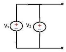
When two ideal voltage sources of emf's V1 & V2 are connected in parallel, what voltage appears across its terminals is ambiguous.
