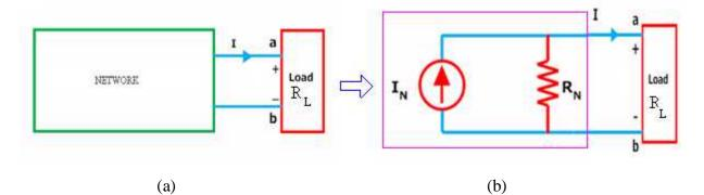
Figure (a) shows a simple block representation of a network with several active / passive elements with the load resistance  $R_L$  connected across the terminals 'a & b' and figure (b) shows the **Norton equivalent circuit** with  $I_N$  connected across  $R_N \& R_L$ .
