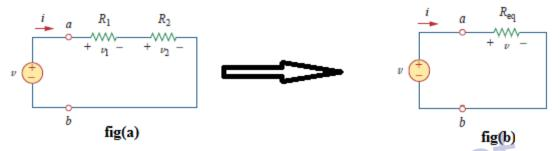
Consider the circuit in fig(a) ,where two resistors  $R_1$  and  $R_2$  are in series, since the same current i flows in both of them. Applying Ohm's law to each of the resistors, we obtain
