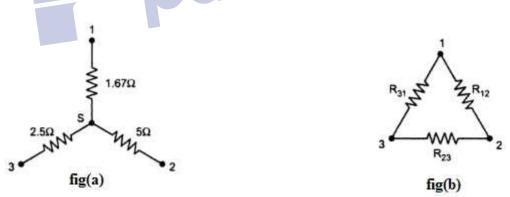
Solution: The equivalent delta for the given star is shown in fig(b), where
