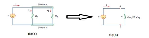
Consider the circuit in fig(a), where two resistors are connected in parallel and therefore have the same voltage across them. From Ohm's law,
