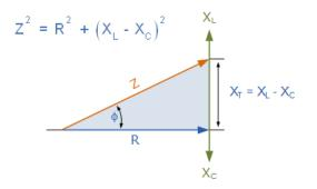
The impedance Z of a series RLC circuit depends upon the angular frequency,  $\omega$  as do X<sub>L</sub> and X<sub>C</sub> If the capacitive reactance is greater than the inductive reactance, X<sub>C</sub> > X<sub>L</sub> then the overall circuit reactance is capacitive giving a leading phase angle.
