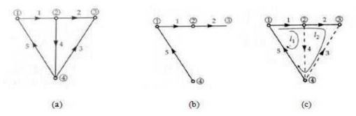
Figure 3: (a) An oriented Graph (b) One of it's Tree (c) The Loops (tie sets) of the Tree
