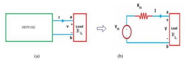
Figure (a) shows a simple block representation of a network with several active / passive elements with the load resistance  $R_L$  connected across the terminals 'a & b' and figure (b) shows the **Thevenin equivalent circuit** with  $V_{Th}$  connected across  $R_{Th} \& R_L$ .
