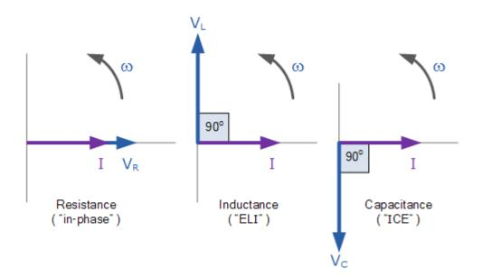
This means then that we cannot simply add together  $V_R$ ,  $V_L$  and  $V_C$  to find the supply voltage,  $V_S$  across all three components as all three voltage vectors point in different directions with regards to the current vector. Therefore we will have to find the supply voltage,  $V_S$  as the Phasor Sum of the three component voltages combined together vectorially.
