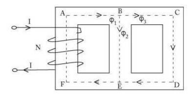
The magnetic paths 'BE' and 'BCDE' are in parallel and form a parallel magnetic circuit. The AT required for this parallel circuit is equal to AT required for any one of the paths. Let  $S_1$ = reluctance of path EFAB
