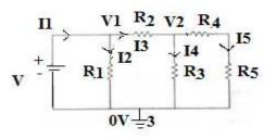
**Step (3):** Apply KCL to those principal nodes for nodal equations and by using ohm's law express the node voltages in terms of branch current.
