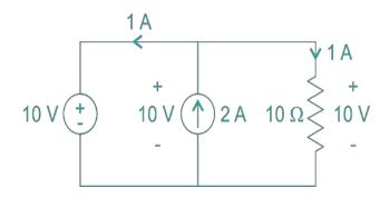
$\therefore$  P<sub>10V</sub> = V. I = 10 × 1 = 10 watt (P<sub>absorbed</sub>).
