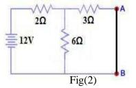
We have shorted the AB terminals to determine the Norton current,  $I_{N.}$  The  $6\Omega$  and  $3\Omega$  are then in parallel and this parallel combination of  $6\Omega$  and  $3\Omega$  are then in series with  $2\Omega$ . So the Total Resistance of the circuit to the Source is:-
