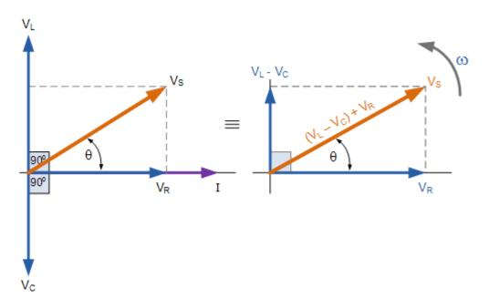
We can see from the phasor diagram on the right hand side above that the voltage vectors produce a rectangular triangle, comprising of hypotenuse  $V_S$ , horizontal axis  $V_R$  and vertical axis  $V_L - V_C$  Hopefully you will notice then, that this forms our old favourite the Voltage Triangle and we can therefore use Pythagoras's theorem on this voltage triangle to mathematically obtain the value of  $V_S$  as shown.
