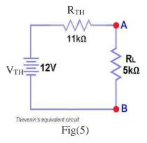
Now apply Ohm's law and calculate the total load current from fig 5.
