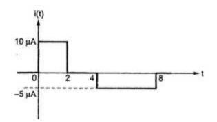
3. A Pure Inductance Of 3mh Carries A Current Of The Waveform Shown In Fig. Sketch The Waveform Of V (t) And P(t). Determine The Average Value Of Power
