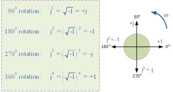
So by multiplying an imaginary number by  $j^2$  will rotate the vector by 180° anticlockwise, multiplying by  $j^3$  rotates it 270° and by  $j^4$  rotates it 360° or back to its original position. Multiplication by  $j^{10}$  or by  $j^{30}$  will cause the vector to rotate anticlockwise by the appropriate amount. In each successive rotation, the magnitude of the vector always remains the same.
