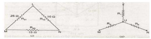
The given circuit thus reduces to the circuit shown in below fig.
