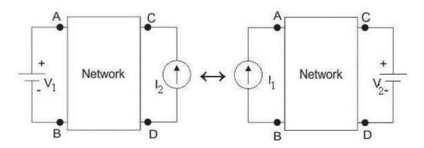
$$\frac{V_1}{I_2} = \frac{V_2}{I_1}$$
