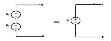
The equivalent single ideal voltage some is given by V= V1 + V2
