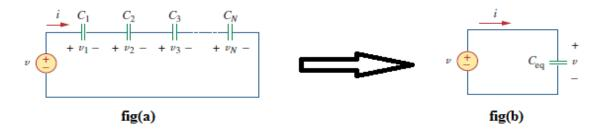
Two or more capacitors in a circuit are said to be in series when the current flowing through all the capacitors is the same.
