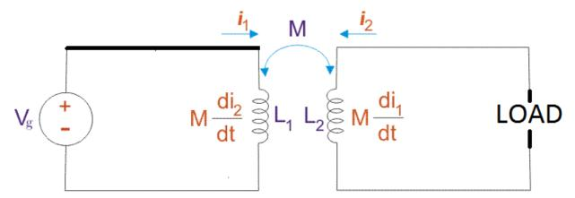
**Mutual inductance** for two coils gives the same value when they are in mutual induction with each other. Induction in one coil due to its own rate of change of current is called self inductance (L), but due to rate of change of current of adjacent coil it gives **mutual inductance** (M)
