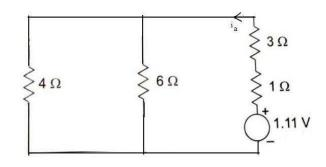
Current due to this additional source of 1.11 V in the 3  $\Omega$  branch  $i_a$  is,
