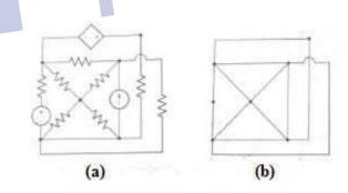
Figure 1: (a) The circuit (b) It's Graph
